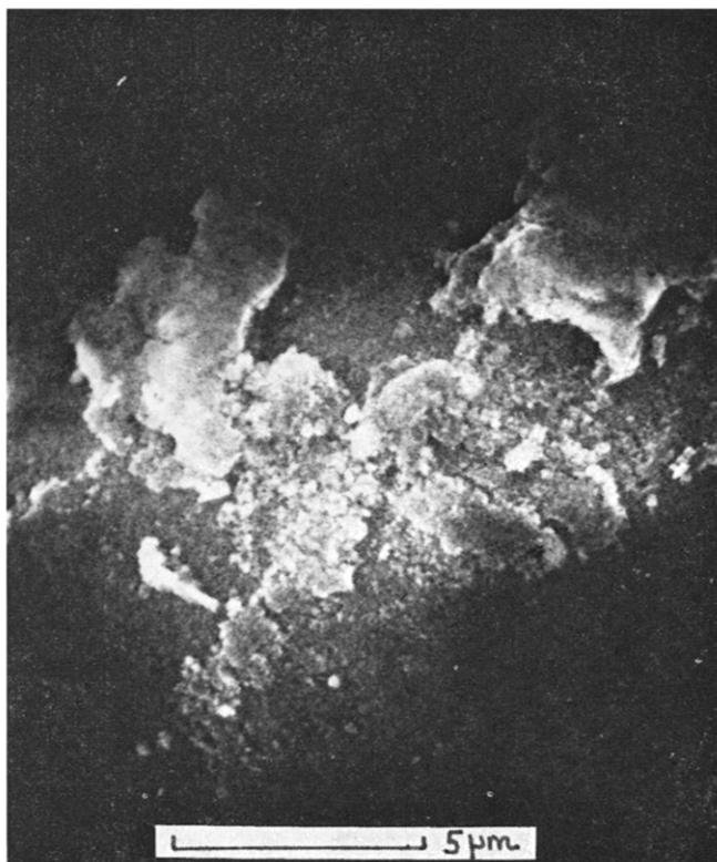
Fig. 2. Detail of a particle of Spherosil coated with 0.84% of pyrocarbon ( cf. , Table I, B).
